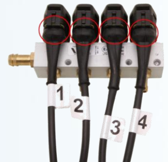
Picture 2t: GAS injectors plugs
