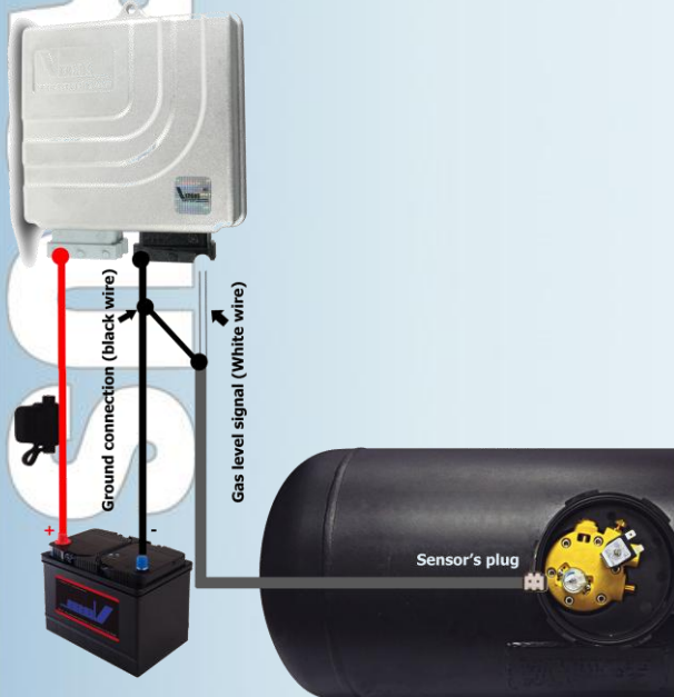
Picture 8b: VERSUS LPG level sensor 1050 type installation scheme
