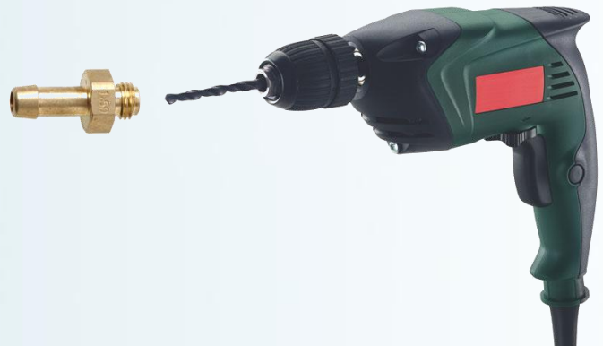
Picture 4j: Drilling the injectors nozzles
