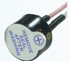
Picture no 9j: Buzzer security label to be removed
